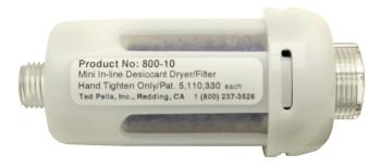
Turns wet dirty air into clean dry air with a four stage filter. 1st stage removes dirt, 2nd stage removes old vapors, 3rd stage removes water vapor, and 4th stage removes residual desiccant dust.
